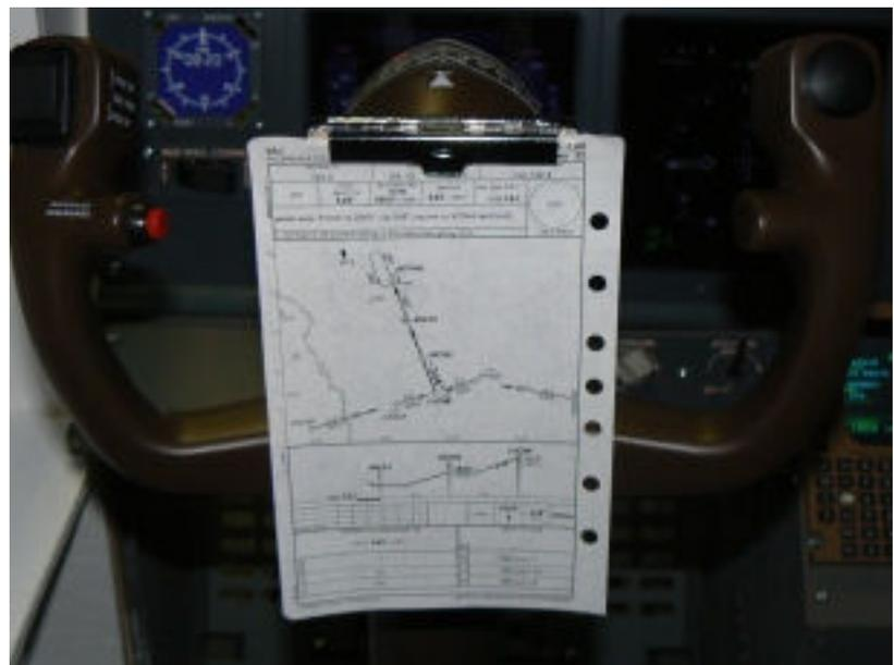
The chart holder on the yoke is sturdily attached with rivets and welds. The clip is of excellent quality and easily holds one or more charts. There is one downfall with this part of the yoke. I found it hard to read the charts when they were clipped to the unit, because the chart holder is mounted flat to the yoke. It would be handy if this chart holder had a bit of an incline to the mount, so the charts would sit on a bit of an angle to make reading them much easier.
