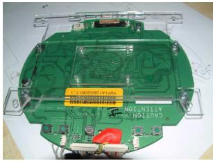
In the above picture you can see four holes in the center of the plexi pieces; these were used to keep the pieces together while the glue settled. There is no space between the plexi and the PCB for the bolt heads or the nuts, so you have to remove them).
