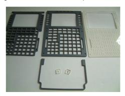
In the rear, from left to right, you see the faceplate, the lightplate, and the backplate or mounting plate, with their protective backing sheets already removed.
