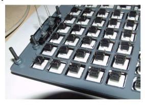
Place the mounting plate on top of the switches. This will need some juggling with switch contacts, but after a few tries every switch contact leg will fall into its designated hole in the mounting plate. No glue needed here!
