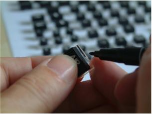
Now first make some plexiglass strips for the annunciator LEDs. I had a piece of 4mm plexi left over, which I also used for the bottom plate which I will describe later. My 1.8mm high-efficiency white LEDs fit nicely into a 2-3mm hole drilled partly into these strips.
