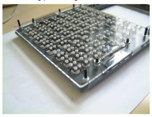
(I first tried this the other way around: lay the mounting plate flat on its back, put the switches into their holes, put all keys on top of the switches, and then try fo fit the face-/lightplate assembly over them – but that actually turned out to be much more difficult. Keys would sag sideways under the lightplate, not fitting into their hole; getting them straightened out with e.g. forceps introduced the risk of damaging the paint on them...).
