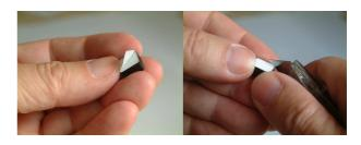
Now we need to glue the keytops and their respective bases together. I did that by first laying the lightplate on top of the backplate, and inserting all key-bases into their holes.
