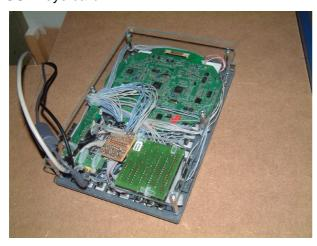
The small ribbon cables at the lower side of the experimenter's board are the connections to the USBKeys card; the bundle of wires at the top side come from the annunciator LEDs. Note: the BRT/DIM buttons go directly to the PCB!
